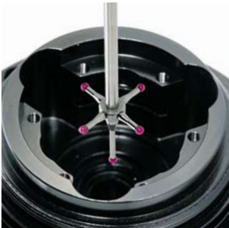
Measuring a complex interior contour
